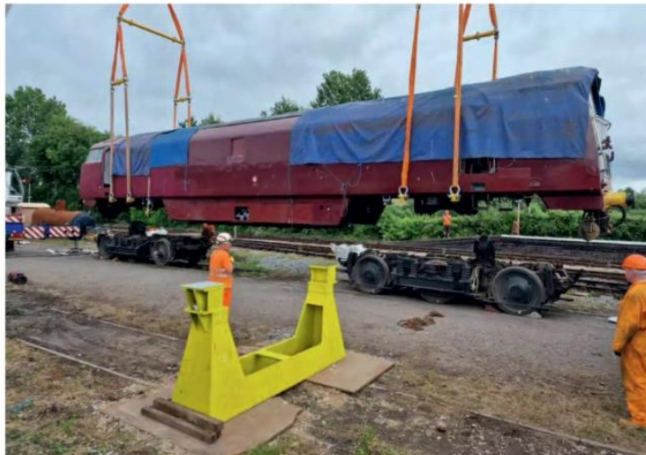
On July 8, Class 52 diesel-hydraulic locomotive D1010 Western Campaigner is lifted clear of its bogies onto one of the yellow ex-Swindon Works locomotive stands in the foreground. Natalie Royal/DEPG
