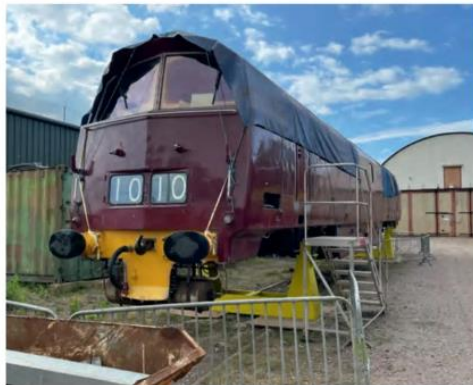
Now situated on locomotive stands in front of the West Somerset Railway's 'Swindon Shed' at Williton, D1010 Western Campaigner will remain here while its bogies are overhauled. Mark Bladwell/DEPG
