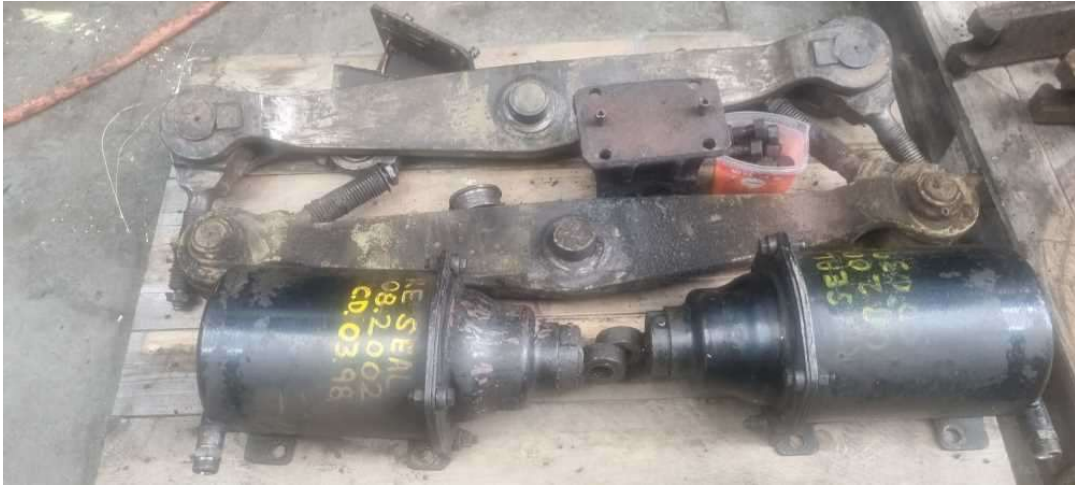
Picture 22 – Brake Cylinders & Equalising Beams
