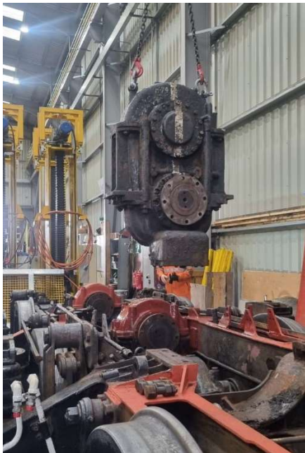
Picture 21 – Intermediate Gearbox Removal
