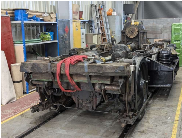
Picture 2 – Bogie Shunt showing wooden sleepers used
