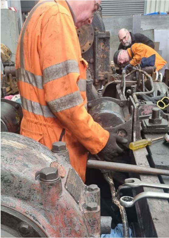
Picture 20 – Brake Cylinder Removal
