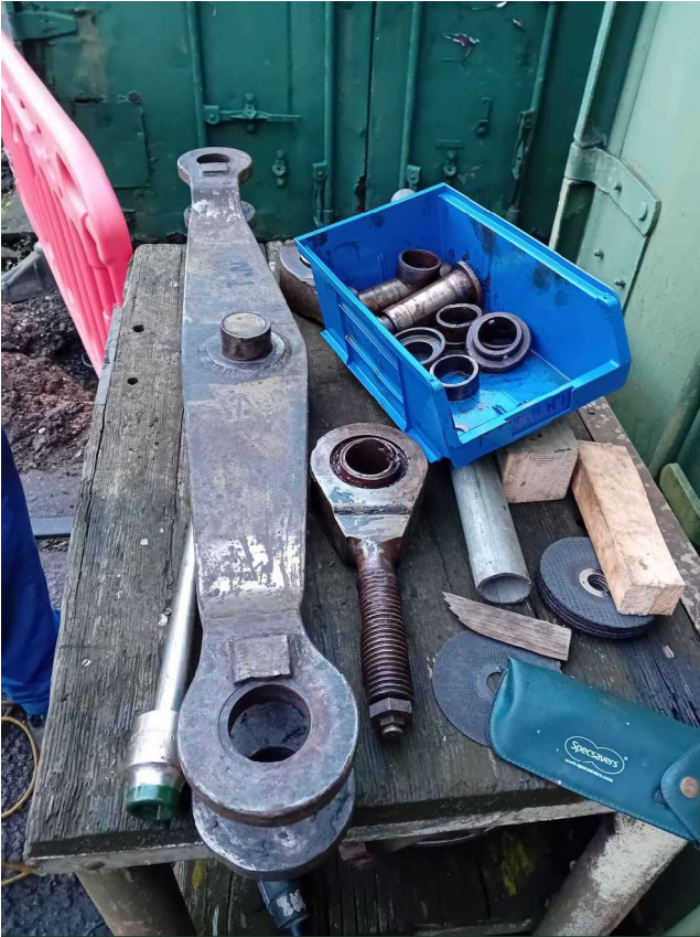
Picture 18 – Equalising Spring Stripped
