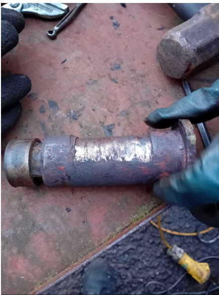
Picture 19 – Equalising Beam Worn
