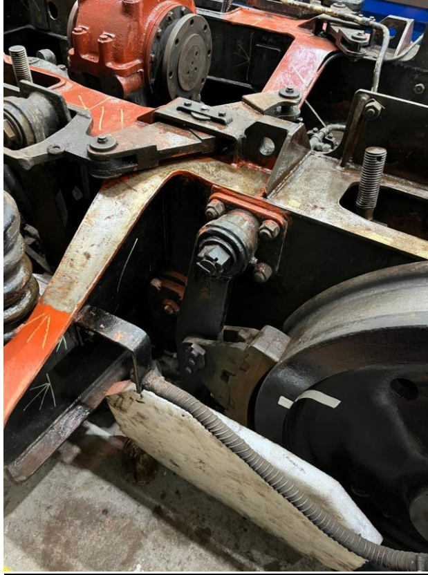
At the end of a cold day's work, "B" end bogie is covered in order to try and keep the damp and condensation out.
