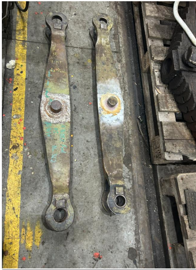
Equalising Beams being prepared for NDT testing – fingers being pointed at areas needing further attention.
