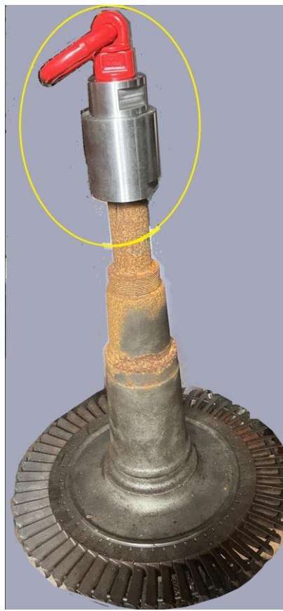
Picture 2 - New Lifting Eye mounted on a spare rotor.
