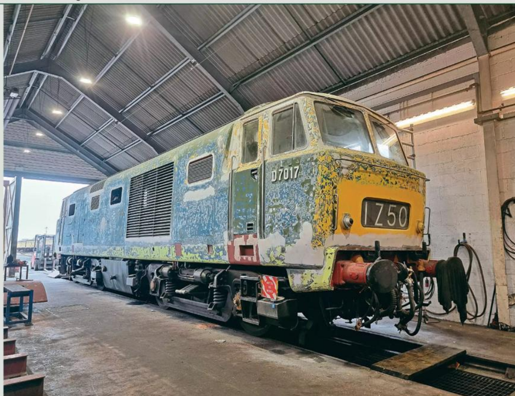
Hymek D7017 has undergone a body overhaul with lots of welding and rubbing down and will appear in early BR blue with small yellow warning panels and light grey window frames. Harry Spencer
