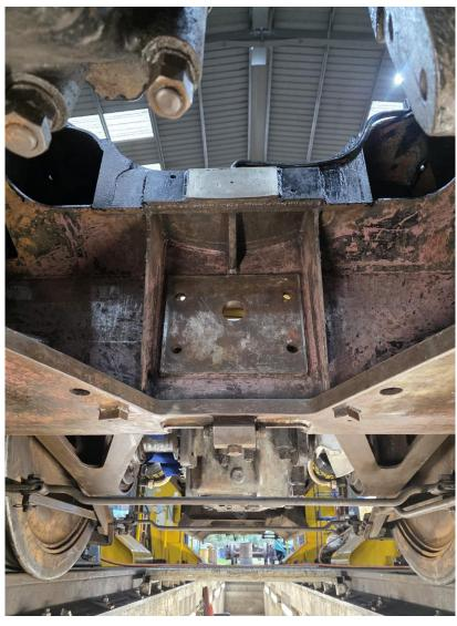
Work also started on the refitting of the lower brake cylinders.
