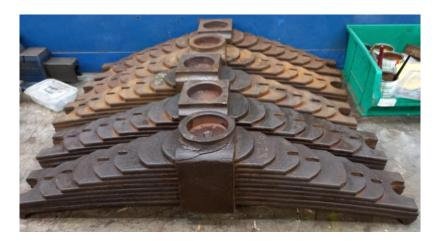
The crack on the first spring is serious, and a new spring will replace this one – we wonder how long D1013 ran with the spring in this condition?
