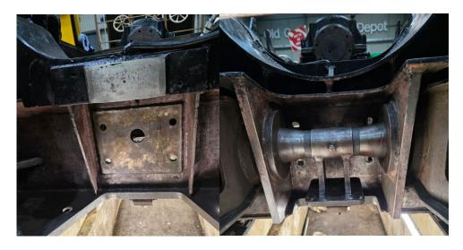
Attention then swung to parts that need cleaning ahead of refitting, pictured below, and the refitting of the torque reaction arms- the centre ones being fitted first.
