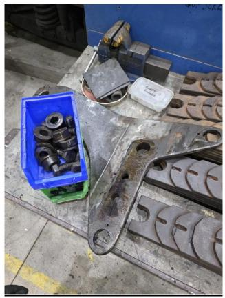
Also of note, the Thrust Pads have been returned from Burton following welding and are ready for refitting.
