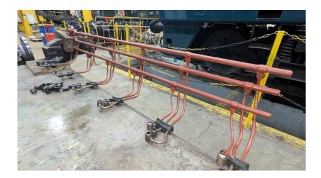
Meanwhile, back to the Torque Reaction Arms with the remaining arms being successfully removed – giving access to the areas above and around them for cleaning ahead of NDT testing.
