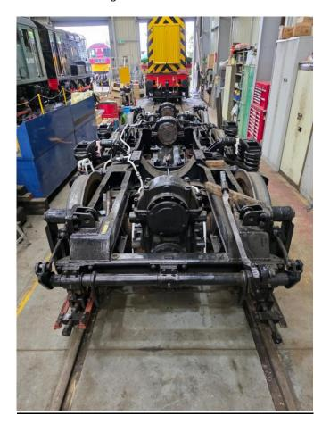
Darren is seen connecting the bogie to the shunt locomotive.
