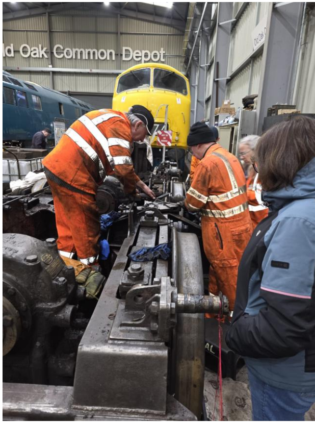
The team removing the thrust brackets and brake rigging from Rangers "A" end.
