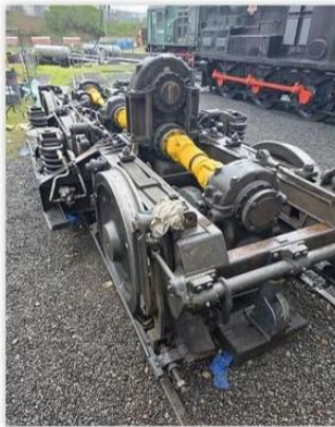
The 'A' end bogie was removed from the locomotive for investigations into a shifted equalising beam, and the opportunity was taken to fit new cardan shafts (yellow). WLA
