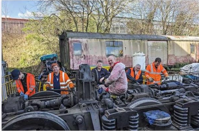
Happiness is... scraping dirt off a Class 52 bogie! Having recently overhauled Western Ranger's 'B' end bogie, WLA volunteers are busy doing the same on the 'A' end bogie. WLA
