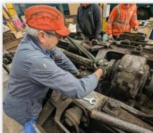
The 'A' end bogie was removed from the locomotive for investigations into a shifted equalising beam, and the opportunity was taken to fit new cardan shafts (yellow). WLA
